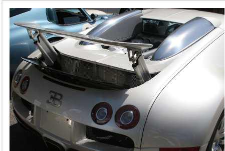
The Bugatti Veyron's hydraulic rear spoiler/air brake in the wing position.
